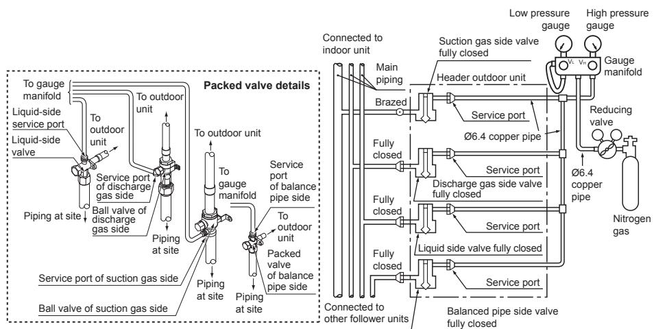
**Able to detect a serious leakage**
