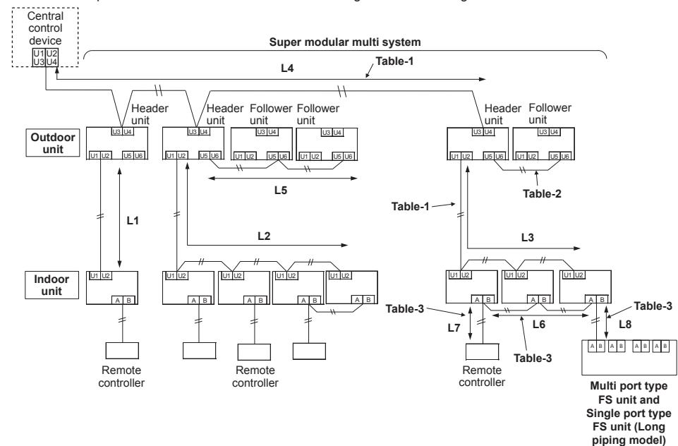
**Table-1 Control wiring between indoor and outdoor units (L1, L2, L3), Central control wiring (L4)**
