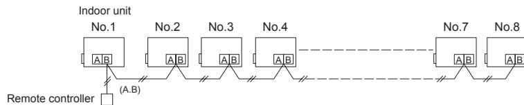
For the group connection within each branch of the Multi port type FS unit and Single port type FS unit (Long piping model) :
