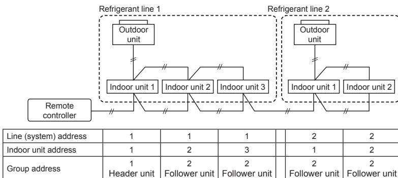
In the example above, disconnect the remote controller connections between the indoor units and connect a wired remote controller to the target unit directly before address setting.
