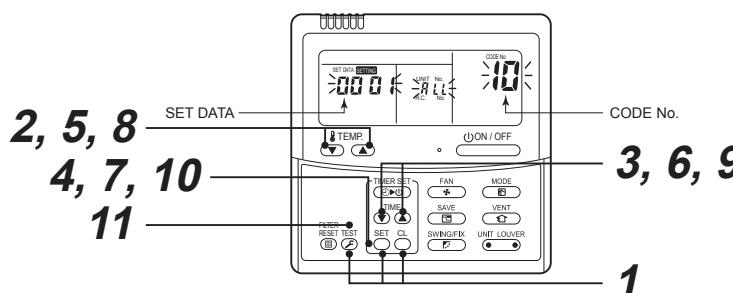
Pair the indoor unit to set and the remote controller one-to-one.
