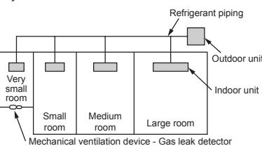
$$\frac{\text{Total amount of refrigerant (kg)}}{\text{Min. volume of the indoor unit installed room (m}^3\text{)}} \leq \text{Concentration limit (kg/m}^3\text{)}$$
