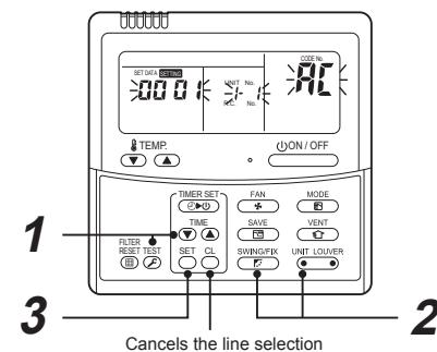
If no number appears on UNIT No., no outdoor unit exists on the line. Push button and select another line following step **2**.
