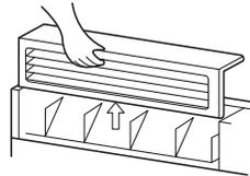
**4 Reverse the air discharge and reattach it to the main unit. Make sure that the four claw hooks (2 at the rear and 2 at the lower sides) are hooked into the mounting positions.**
