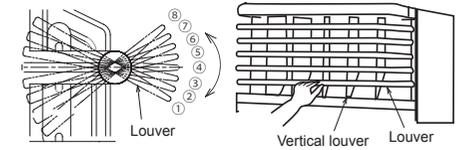
The louvers can be adjusted at 8 phases linking with 5 louvers. When changing the louver angle, hold near the center of louver and move it slowly.
