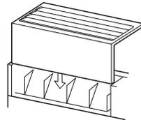
**5 Be sure to tighten the air discharge with the removed fixing screws so that it does not come off.**
