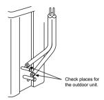
· Check the flare nut connections for the gas leak with a gas leak detector
